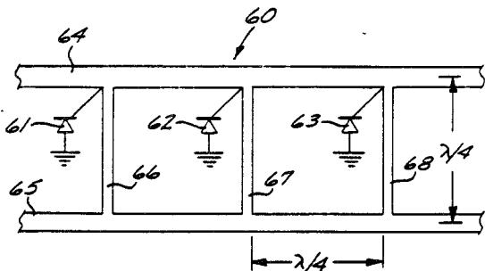
**Integrated Optical Waveguide Polarizer**
